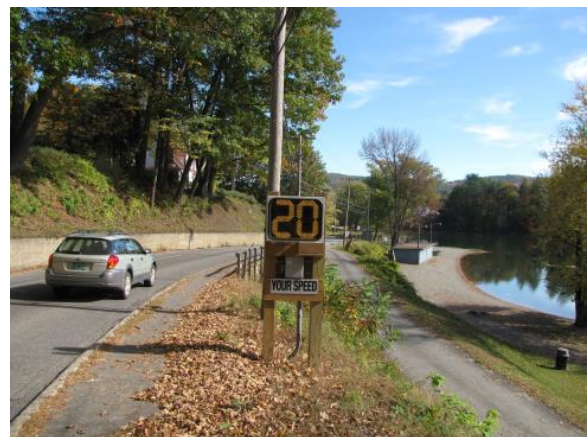
The recently installed speed feedback sign monitors motorists on Ascutney Street near the Mill Pond
